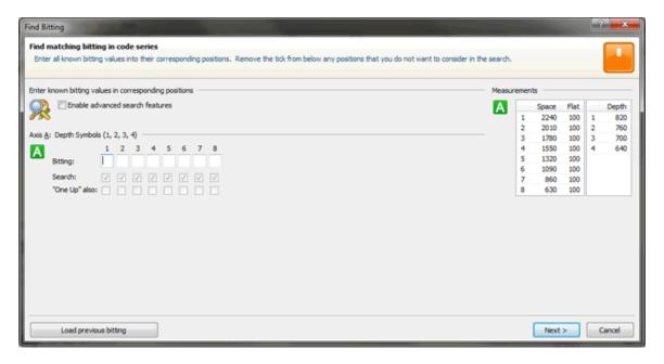
Type in the bittings that you can read off the damaged key...
